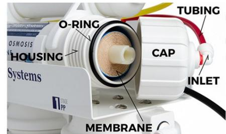
1. The RO membrane typically lasts about 2 – 3 years. The membrane life span depends on the source water quality, your water usage, and how often the three pre-filters are replaced. To ensure the system's performance and water purity, it is important to replace the pre-filter cartridges on schedule. Use a TDS meter to periodically to check the RO water purity.
