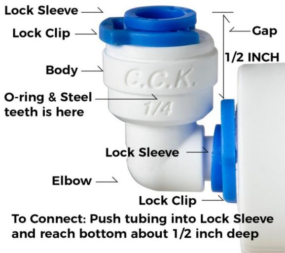
To Connect: Push tubing into Lock Sleeve and reach bottom about 1/2 inch deep
